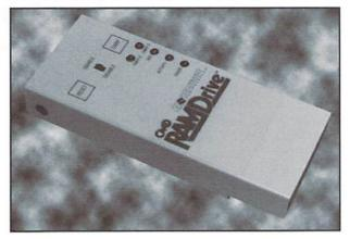
and blackout protection, the RAMDrive features internal rechargeable nicad batteries. The unit features CMD's transparent DOS interface, and with the use of a cartridge port expander can take advantage of REU's. Like the RAMLink, the RAMDrive features a number of LED's to reflect its current state.
