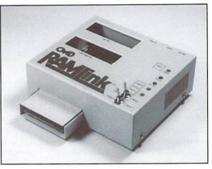
RAMLink disable switch. In the back of the RAMLink unit rests a parallel port, offering CMD HD Series hard drive owners faster access. The RAMLink comes standard with a small power supply and has a battery backup option. Both of these plug nicely into the back of the cartridge. And finally, the RAMLink features a number of LED's to reflect its current state.
